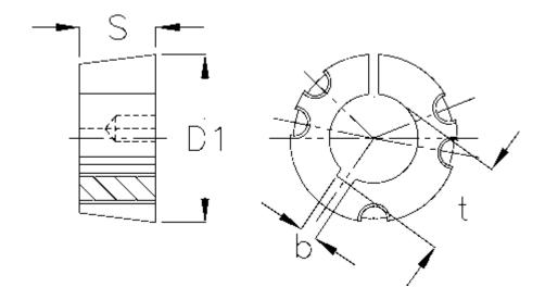
$\begin{array}{lll} b & = 14 \\ Bore & = 48 \\ Bush type & = 4030 \\ D1 & = 146 \\ S & = 76,2 \\ Screw size & = 5/8 \times 1 \ 1/2" \\ t & = 51.8 \end{array}$
